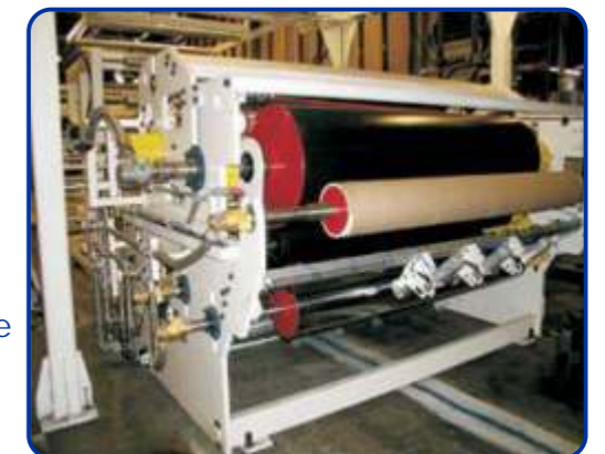
Third Layer Lamination Station
